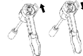
The handheld pendant switch activates a solenoid that activates power to the winch motor. To connect the pendant control, remove the cover on the plug receptacle and insert the plug end of remote switch. The plug on the pendant control cord is keyed and will fit into the socket only one way. The switch trigger returns to the "Off" position when released. To change direction, move the toggle in the other direction.
