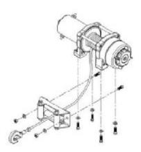
in order to make sure the motor, drum and gearbox housing are aligned correctly.
